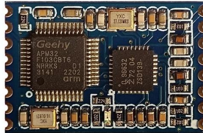
Core Module with MCU APM32F103CBT6
