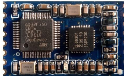
Core Module with MCU GD32F350CBT6
